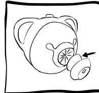
\* The air mesh is there to prevent solid objects and dust from entering the housing.
